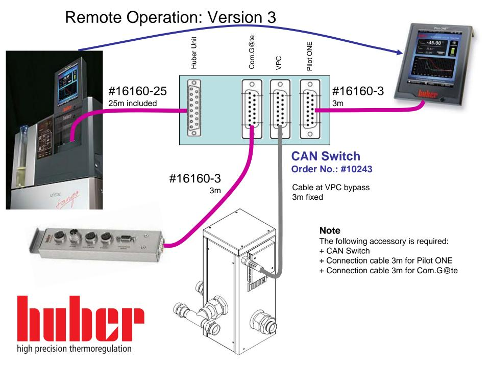
Remote Operation: Maximum lengths for spec. **Huber Unit** Pilot ONE VPC #16160-x #16160-x 3m to max. 50m 3m to max. 50m **CAN Switch** Order No.: #10243 #16160-x Cable at VPC bypass max. 10m 3m fixed **Note** The maximum possible cable lengths are specified. Special lengths are available on request. high precision thermoregulation
