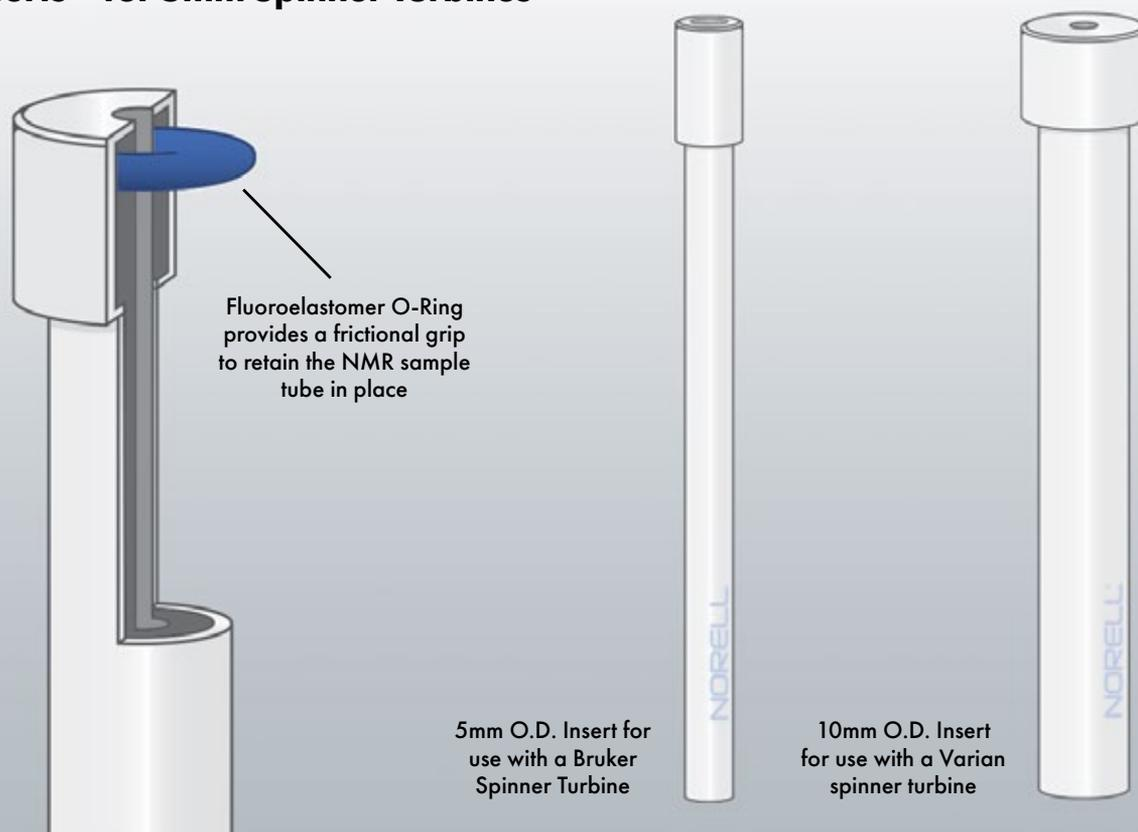
Precision adapter, made from a proprietary formulation of acetal homopolymer resin, holds 1.5mm, 1.7mm, 2.0mm, 2.5mm, 3mm, 4mm or 4.25mm NMR tubes in 5mm spinner turbine. Available for Agilent/Varian, Bruker & Jeol spectrometers. Does not include spinner turbine. U.S. Patent #7,728,593.
