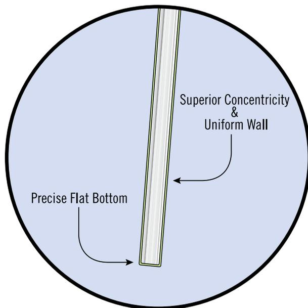
Through our advanced manufacturing process, the NMR tube bottoms are uniformly hemispherical and consistent, thereby minimizing shimming and susceptibility differences among samples. This uniformity extends throughout the wall thickness of the tubes, maximizing the concentricity among tubes and lots. This translates to more consistent placement of the contained sample volumes in today's advanced, highly homogeneous, high field NMR magnets.
